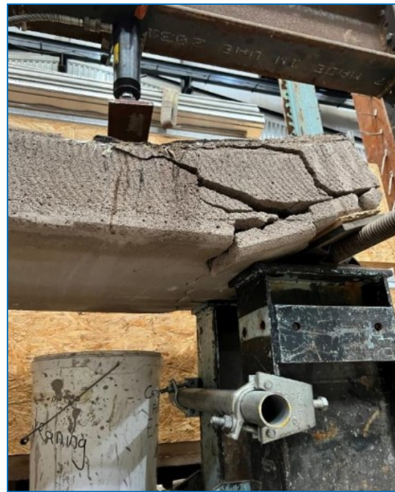
Figure 3 - Laboratory Setting of Compressive Strength of RAAC panel end bearing. Source Loughborough University
