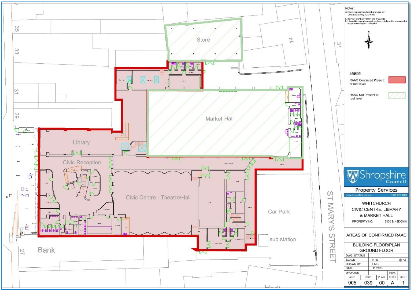
Figure 12 - Whitchurch Library & Civic Centre – Ground floor areas of confirmed RAAC at roof level.
